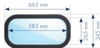
Rounded corners ( r = 100 \text{ mm} ), excellent insulative value
