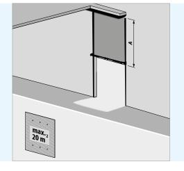
T 500 hF vertical rail system with low spring axis + steel support profile A = open height + 400 mm, B = n/aWidth max. 4,500 mm
