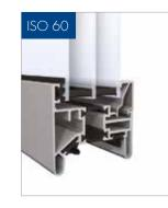
Panorama door 60 mm Triple Plexiglas Optical 40 mm (4-14,75-2,5-14,75-4 mm) **U-value of the Panoramic door 60:** 4,000 x 4,000 mm: 2.45 W/m<sup>2</sup>K
