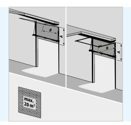
T 400 hF elevated rail system with low spring axis + steel support profile
