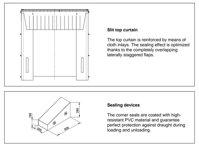
The advantage for the mechanical dock shelter type PMSK
