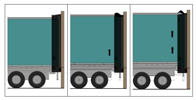
The vehicle is lifted after dock-in into the dock shelter. The roof automatically follows this movement and returns to its original position after the vehicle has left the docking station.
