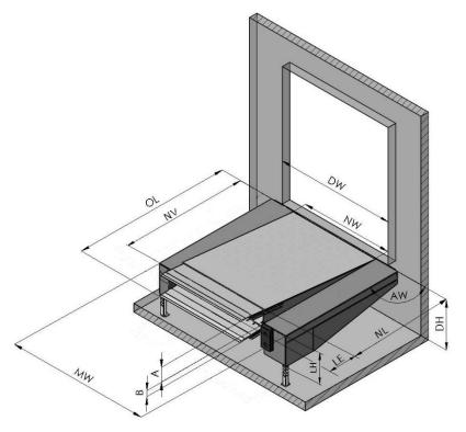
In accordance with the EN 1398 standard, the leveller must not be used beyond the permissible gradient range of  $\pm$  12.5% (around  $\pm$  7°). The limits may only be exceeded if the operator ensures that the danger of slipping has been eliminated (e.g.: due to dry and clean surfaces).
