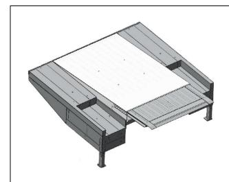
The stepped version of the loading ramp is used when the lorry docks in with its rear doors closed; the doors are opened only after completion of the dock-in process. Compared to the leveller platform, the areas on the left and on the right side of the dock leveller are lowered by 300 mm over a length of 1200 mm or 1300 mm, i.e. over the width of the lorry doors.
