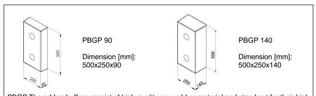
PBGP The rubber buffers consist of high-quality new rubber material and stand out for their high resistance to wear and tear; they are available in two different versions.
