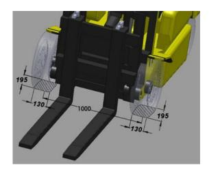
The integrated PT2 telescopic lip leveller is provided with the CE and meets all requirements of the EN 1398 standard. The standard load capacity of 100 kN (dynamic axle load) corresponds to the EN 1398 standard for a forklift wheel contact surface of 130x195 mm. Higher concentrated loads as well as higher load capacities are available on request at short notice.
