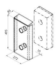
PZPS 90 07 With protective housing (3-side frame), hot-dip galvanized, for rubber buffer PGF 90
