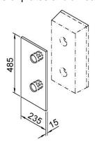
PZPS 140 01 Front protection plate (hot-dip galvanized) for rubber buffer PGF 140
