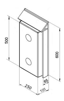
PGFS 140 Rubber element (thickness 140 mm) with protective housing
